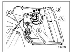
7.14 Press the retaining lugs on the rear light cluster bulbholder together (broken arrows) to release the bulbholder
